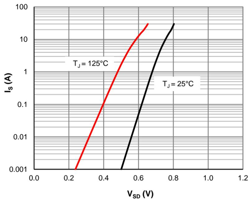
**Figure 7: Body-Diode Characteristics**
