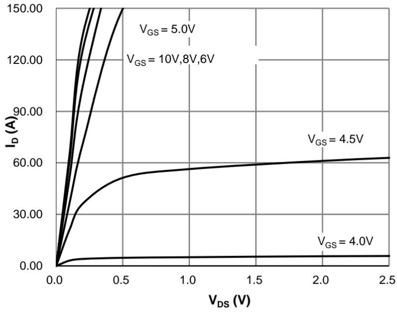
**Figure 1: Saturation Characteristics**
