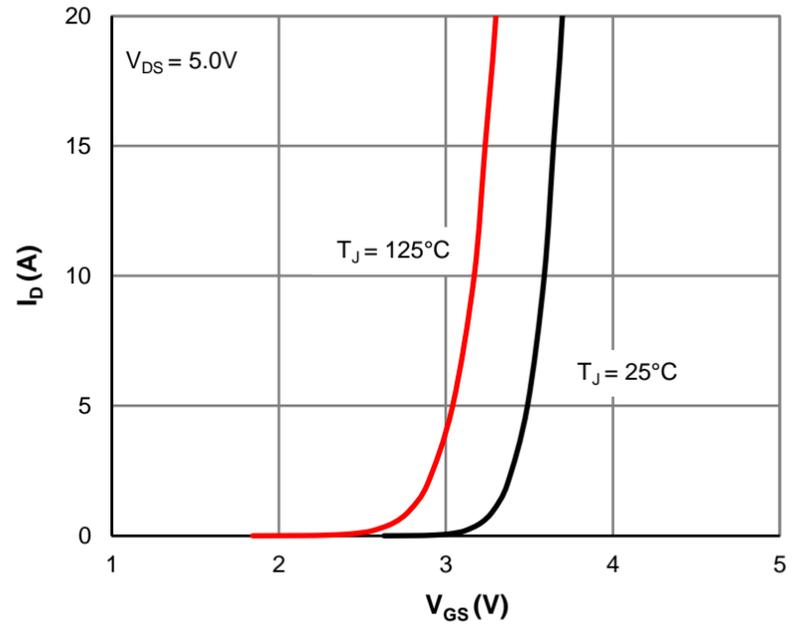
**Figure 2: Transfer Characteristics**
