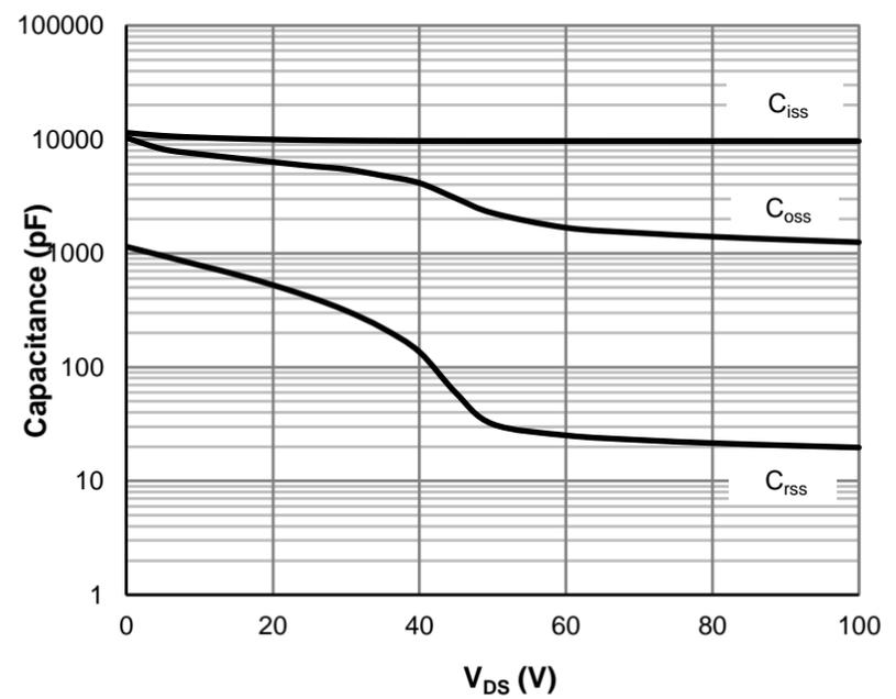
**Figure 8: Capacitance Characteristics**
